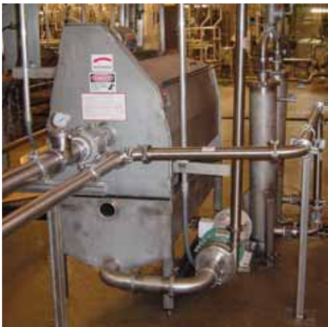
Self Cleaning Screen and cleaned on the fly filters.
